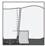
3. Line up one piece of tape with the mark and with space in between foam panels, and press onto side foam panel.
