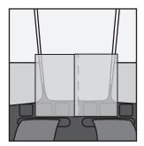
Center foam panel: align final tape with top of harness slot and second rib from outside and press into center foam panel.
