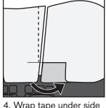
4. Wrap tape under side foam panel and press to secure.
