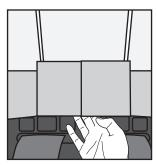
Center foam panel: wrap both tape pieces under center foam panel and press to secure.
